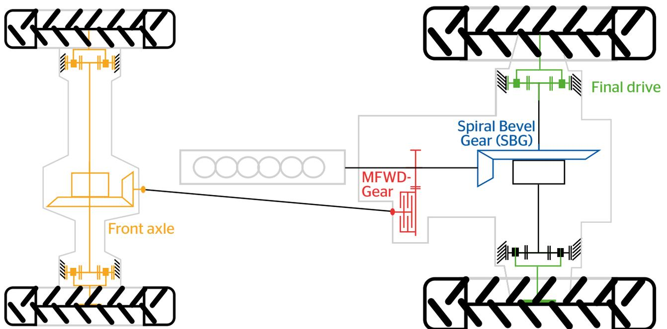
If "R" is not defined, because the tractor is available in many different ratio combinations, it can be calculated with the values shown in the picture, if this information is available in tractor handbook or on ID plates of transmission and front axle.
